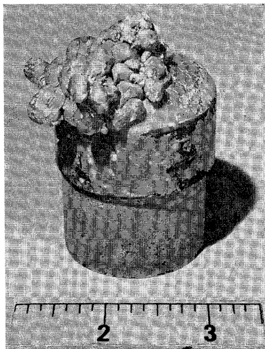
Fig. 11 Expansion of the salt mixture resulting from the release of dissolved gases when the salt was cooled rapidly.
